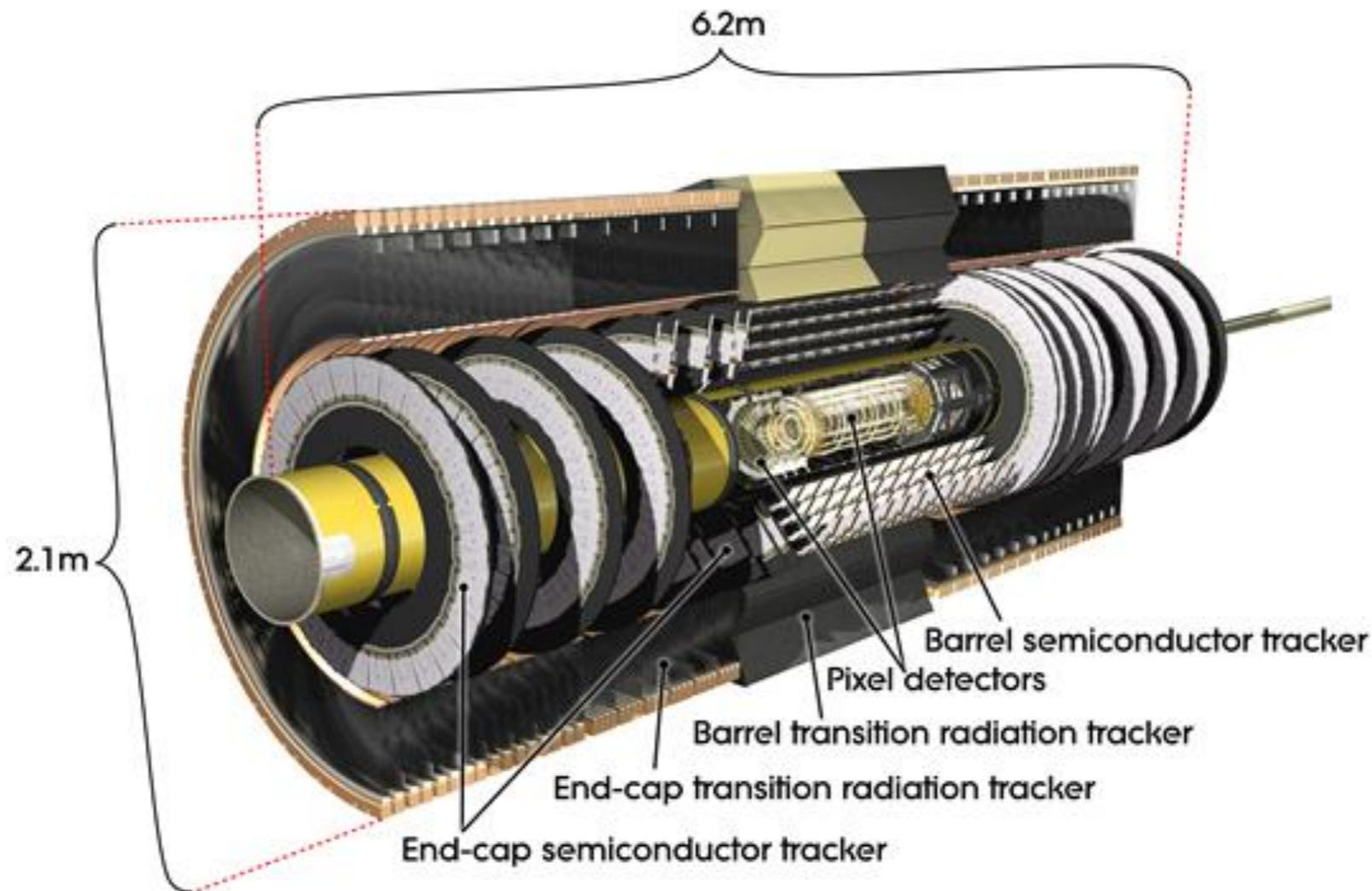
The inner detector of ATLAS sees charged particles and measures their momenta in Pb+Pb collisions at 5.02 TeV
