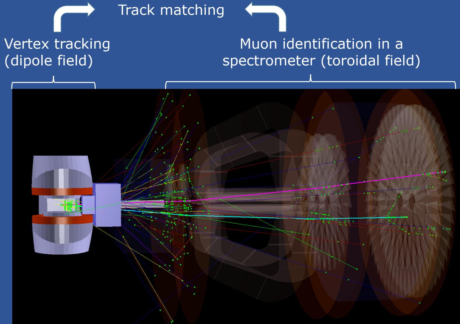
Track matching: measure muon kinematics before multiple scattering and energy loss
